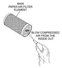
Figure 20. Cleaning Paper Air Filter Element
